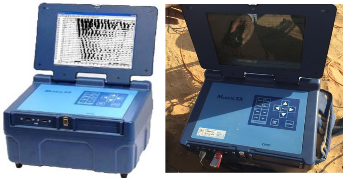
Fig (3): McSEIS-SX 24 channels Seismograph during the field survey at the study area
